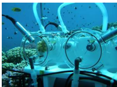
Incubation chamber used to measure metabolic rates of corals. Developed by Yvonne Sawall and built by the workshop at GEOMAR.
