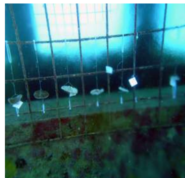
Fungia granulosa exposed to highly increased salinities in the discharge screen of the KAUST seawater reverse osmosis desalination plant during the 29 day experiment.
